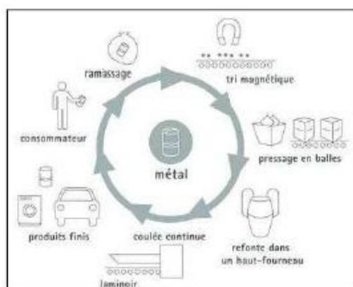
Figure 1 : Recyclage des structures porteuses
