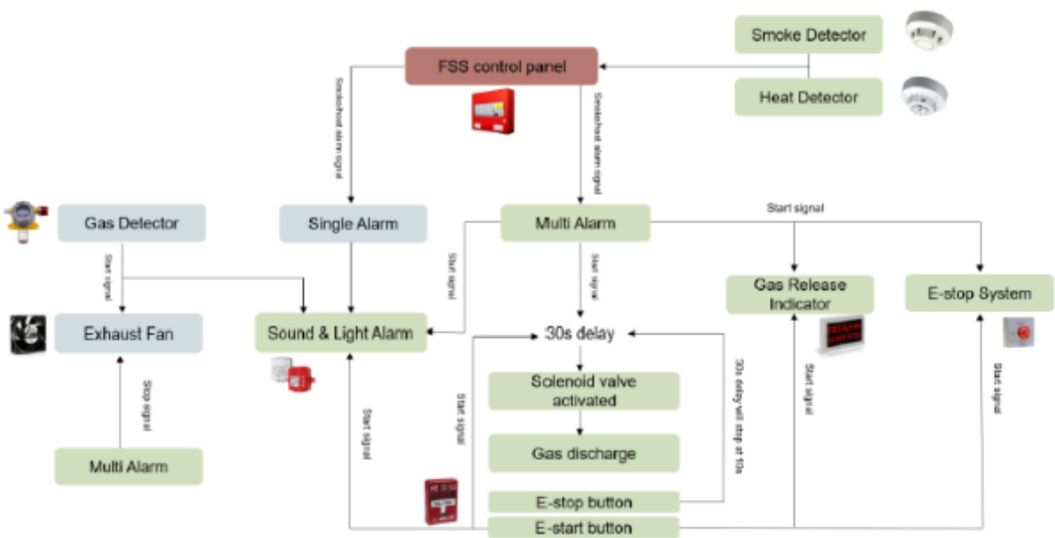
Figure 4-3 Fire Suppression System Work Flow (For reference)
