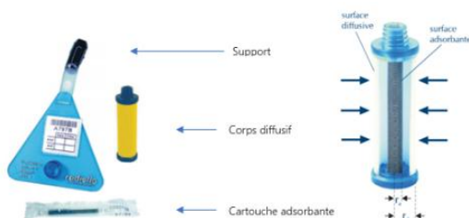
Figure 32 : Echantillonneur passif Radiello
